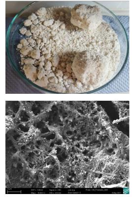
SEM-picture CSH development with high pore volume and specific surface area
